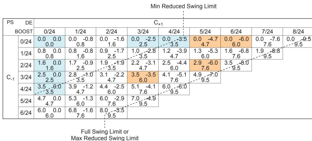
Figure 8-9 Transmit Equalization Coefficient Space Triangular Matrix Example
