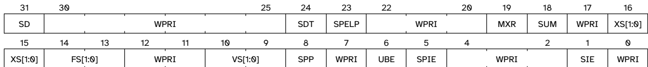
Figure 98. Virtual supervisor status ( vsstatus ) register when VSXLEN=32 .
